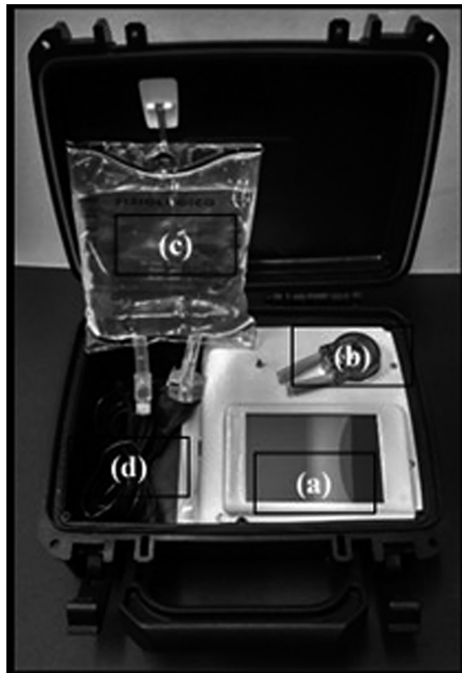
Figure 1. Autonomous infuser: screen (a), pump (b), saline solution (c) and electrical cord (d).
