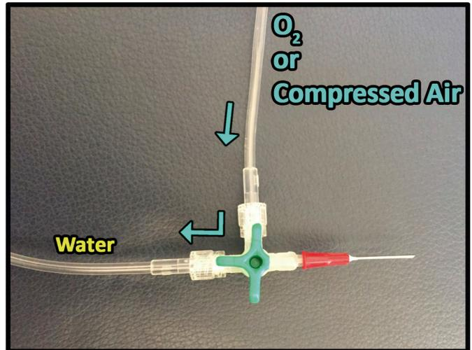
Figure 4. A 3-way stopcock opens the pathway between the compressed air supply and the bottle containing distilled water.
