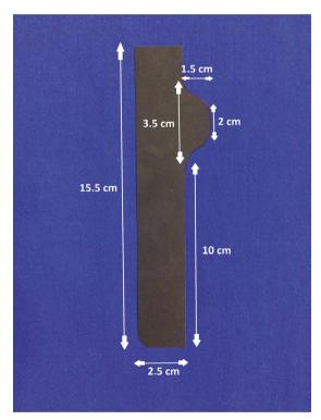
Figure 1. Measurements of the mold.
