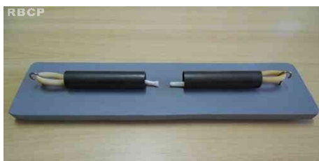
Figure 2 - The simulator fitted with swine tendons already in place.
