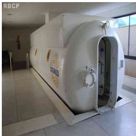
Figure 1 - Hyperbaric chamber gradually increases ambient pressure and maintains it without variation at the hyperbaric level during the duration of the treatment.
